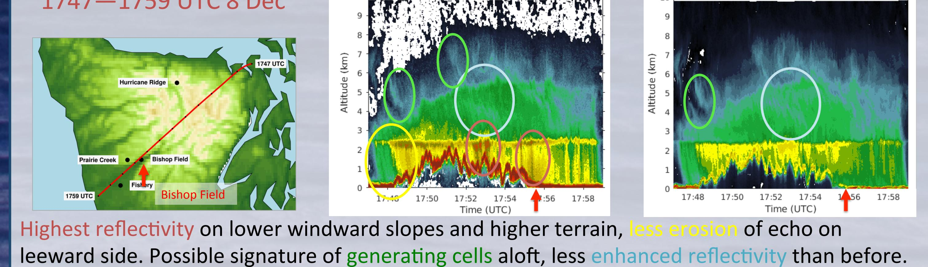
Highest reflectivity on lower windward slopes and higher terrain, less erosion of echo on leeward side. Possible signature of generating cells aloft, less enhanced reflectivity than before.
