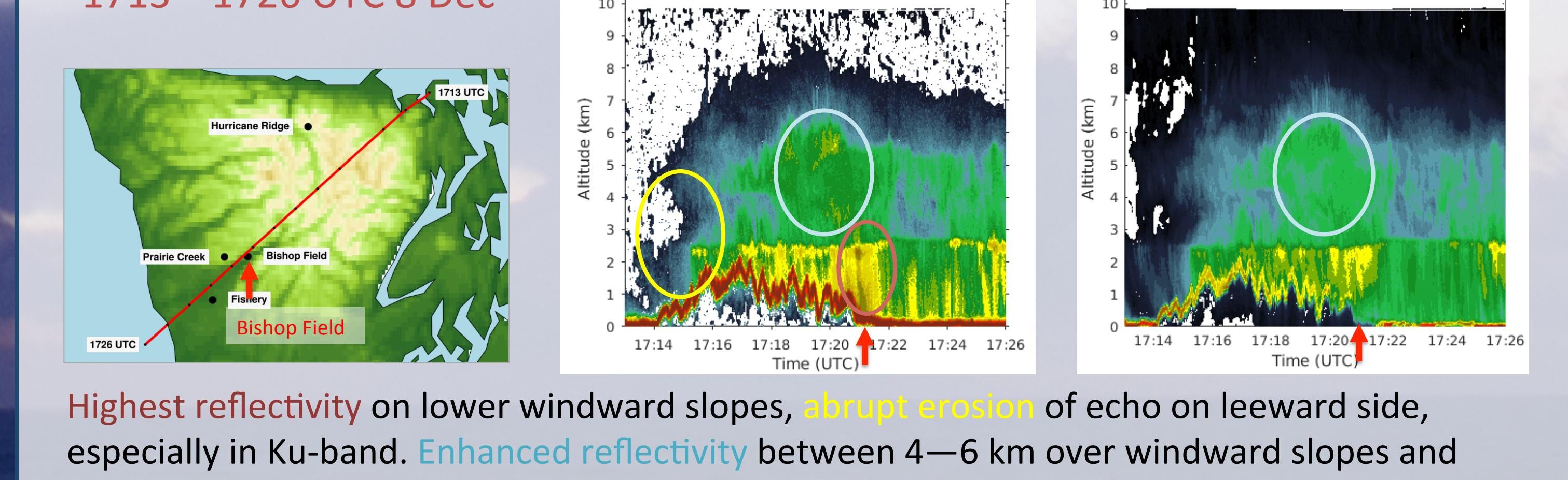
Highest reflectivity on lower windward slopes, abrupt erosion of echo on leeward side, especially in Ku-band. Enhanced reflectivity between 4–6 km over windward slopes and high terrain.
