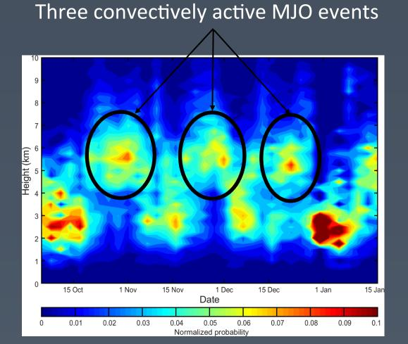
Top: Normalized probability of detection of 20 dBZ echo top for convective echoes composited between 3°N, 9°N, 68°E, and 78°E. 25–30 day variability in modal distribution is observed.
