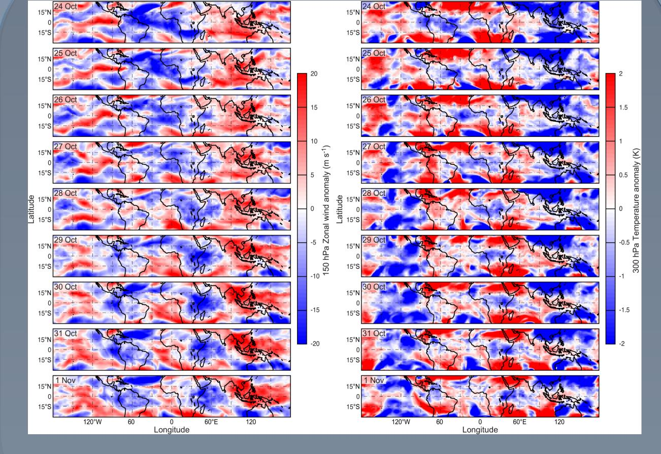
Left: 150 hPa u'. Right: 300 hPa T'. As large-scale anomaly of one sign propagates into Indian Ocean, it is confined to near equator at first. Anomaly spreads meridionally as wave becomes coupled to convection.
