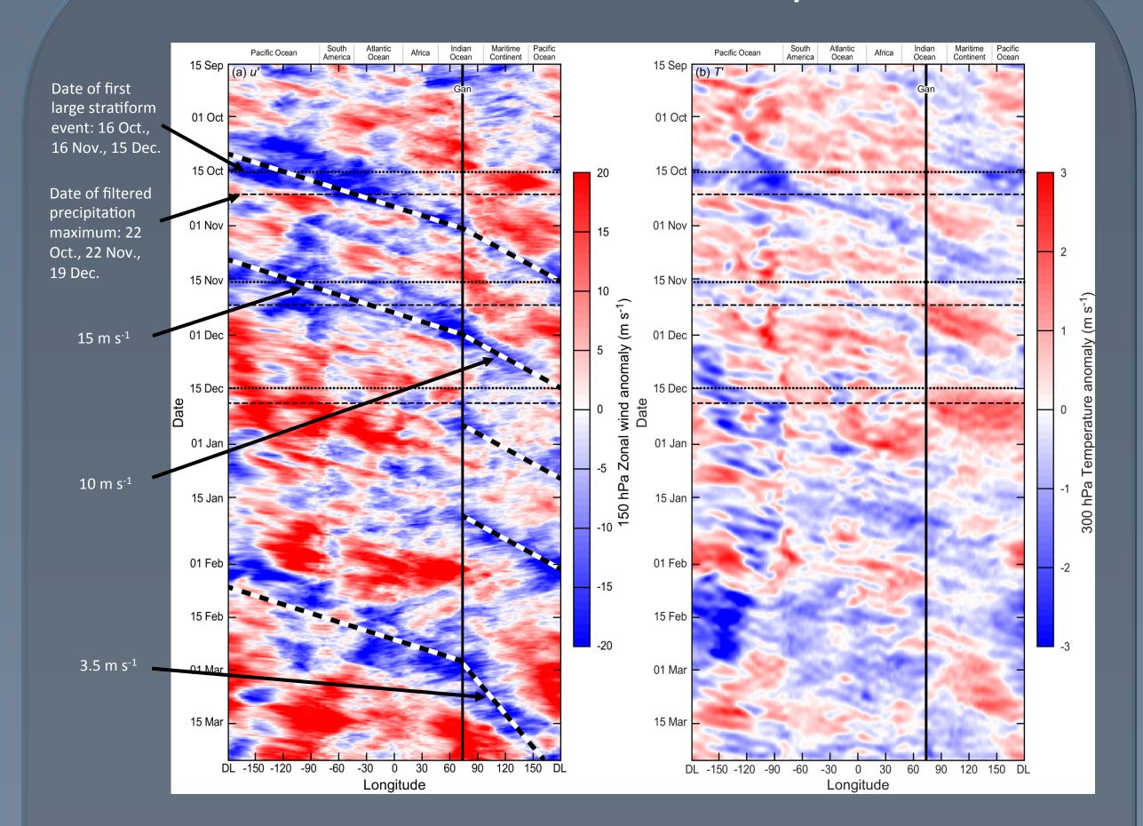
Left: Hovmöller for 150 hPa u anomaly. Right: Hovmöller for 300 hPa T anomaly. Easterly propagating anomalies of zonal wind and temperature move into Indian Ocean. Convective outbreak does not begin until divergent anomaly appears at 150 hPa. Propagation speed and relationship between structures of u' and T' confirm a Kelvin wave. Signal propagates more slowly eastward after convection is coupled to wave. T' is more in quadrature with u' after coupling, a signal of a forced Kelvin wave.
