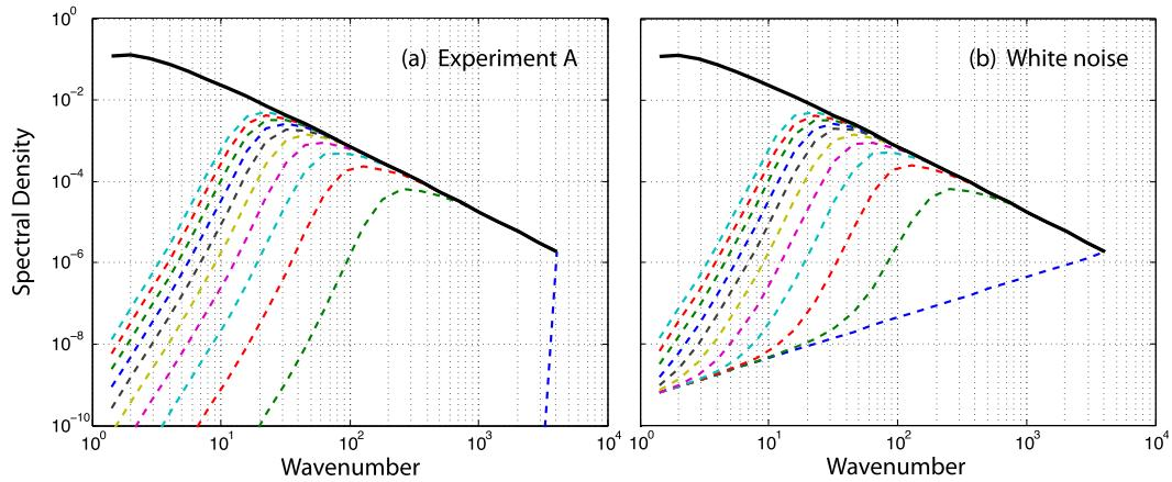
FIG. 2. KE' spectral density  $Z_k/k$  as a function of wavenumber  $k$  at nondimensional times  $t = 0, 0.1, \dots, 1.0$  for initial error saturated at the largest wavenumber and (a) zero elsewhere and (b) following a white-noise spectrum. These and subsequent calculations are performed using 24 modes with  $\rho = \sqrt{2}$  and a smooth approach to nonlinear saturation.
