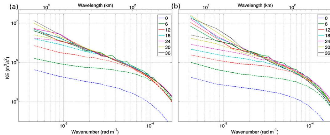
FIG. 4. Ensemble- and meridional-averaged total (solid lines) and perturbation (dashed lines) kinetic energy spectra at 500 hPa shown every 6 h (line colors given in the legend) for the COAMPS ensemble initialized (a) 1200 UTC 4 Feb and (b) 1200 UTC 25 Dec 2010. Only those wavelengths greater than  $7\Delta x$  are shown; the spectrum for the initial  $\widehat{KE}$  is omitted.
