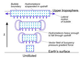
**Figure 4** Conceptual model of a buoyant updraft element. Dots indicate hydrometeors suspended by updraft; downward-pointing arrows indicate particles heavy enough to fall through updraft; horizontal arrows indicate lateral spreading of bubble. Open arrows represent the vector field of the buoyancy pressure gradient force (From Yuter and Houze, 1995c. Reprinted with permission from the American Meteorological Society.)
