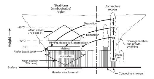
**Figure 9** Schematic of the precipitation mechanisms in a mesoscale convective system. Solid arrows indicate particle trajectories. (From Houze, 1989. Reprinted with permission from the Royal Meteorological Society.)
