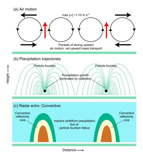
**Figure 5** Conceptual models of vertical cross sections through idealized young, vigorous precipitating convection with no environmental shear. (From Houze, 1997. Reprinted with permission from the American Meteorological Society.)
