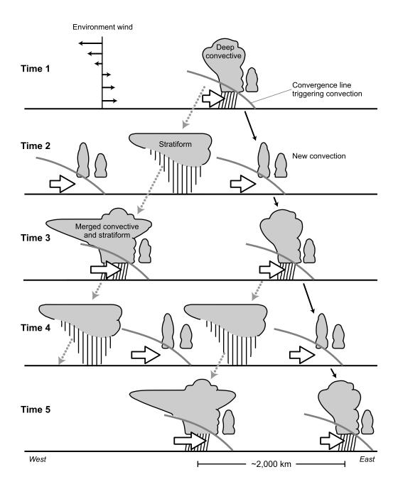
**Figure 10** Schematic of convective evolution over the near-equatorial Indian Ocean. An eastward moving convergence line triggers convection, and lower tropospheric winds advect the new boundary-layer rooted convection eastward. Upper-level winds advect the stratiform cloud and precipitation formed as the convection matures to the east, where it intercepts new convection formed to its west. (Adapted from Yamada et al. 2010. Reprinted with permission from the American Meteorological Society.)
