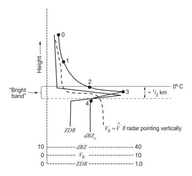
**Figure 2** Schematic of vertical profile of radar data in stratiform precipitation. Solid curve shows reflectivity. Dashed curve shows Doppler radial velocity  $V_R$  with the antenna at vertical incidence. Under stratiform conditions  $V_R$  is related approximately to the mass-weighted terminal fall speed of the particles,  $\hat{V}$ . Points 0-4 bound the layers in which different microphysical processes dominate (see text for further discussion).
