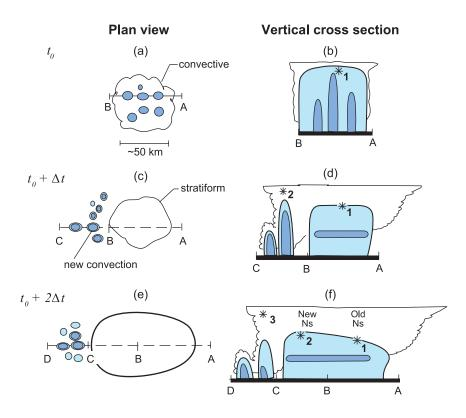
**Figure 7** Conceptual model of the development of nimbostratus associated with deep convection. Panels (a), (c), and (e) show horizontal radar echo pattern at the earth's surface with two levels of intensity at three times,  $t_o$ ,  $t_o + \Delta t$ , and  $t_o + 2\Delta t$ . Panels (b), (d), and (f) show corresponding vertical cross sections. A sketch of the visible cloud boundary has been added to the vertical cross sections. Asterisks trace the fallout of three ice particles.
