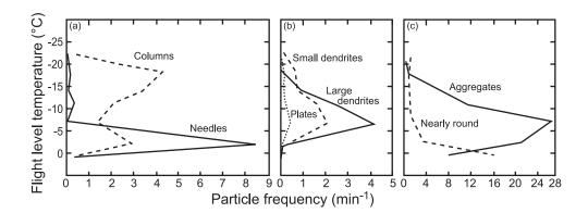
**Figure 3** Ice particle data obtained on aircraft flights through nimbostratus in tropical mesoscale convective systems over the Bay of Bengal. Plots show relative frequency of observation of ice particles of a particular type per minute of in-cloud flight time as a function of flight-level temperature. (From Houze and Churchill, 1987. Reproduced with permission from the American Meteorological Society.)
