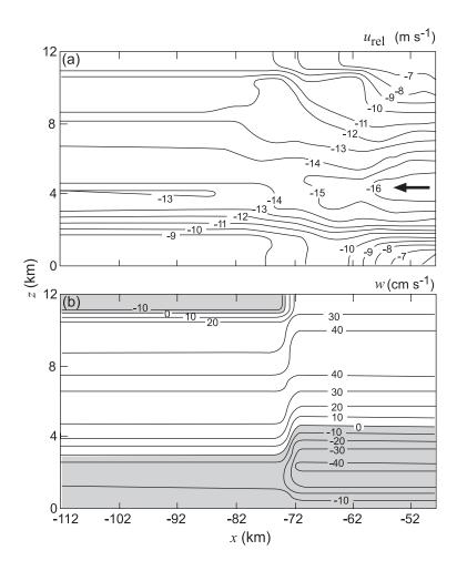
**Figure 11** Horizontal wind and vertical air motion assumed to exist in the domain of a numerical simulation of a stratiform region. Deep convection is assumed to be located immediately to the right of the domain. Data are from a squall-line mesoscale convective system observed over Oklahoma. (From Rutledge and Houze, 1987. Reprinted with permission from the American Meteorological Society.)
