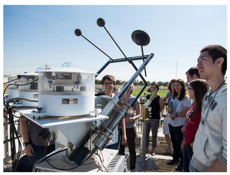
The inaugural atmospheric research instrumentation class at the Pacific Northwest National Laboratory toured the Atmospheric Measurements Laboratory's "skystand" platform, which includes a group of radiometers measuring solar energy at different angles. Credit: Andrea Starr, PNNL
