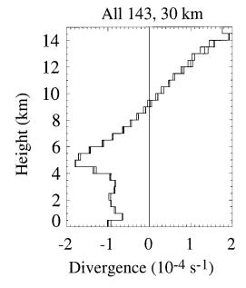
Fig. 7. Mean of all divergence profiles measured by airborne Doppler radar in tropical precipitation over the western tropical Pacific during TOGA COARE. The average is based on 143 samples, obtained on 10 different aircraft missions. [From Mapes and Houze (1995).]
