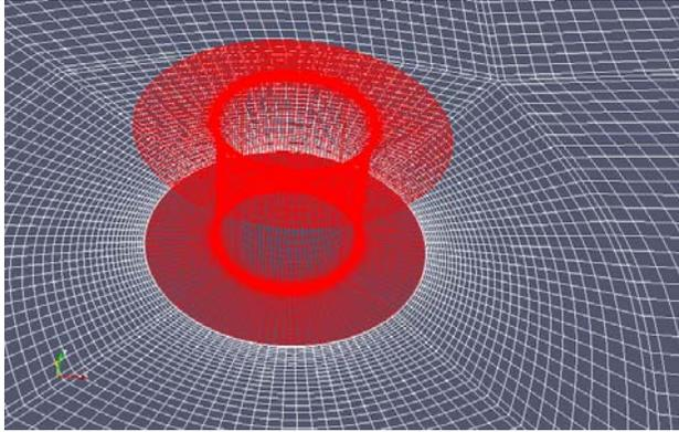
**Figure 10.** Details of the multi-block, non-orthogonal mesh.
