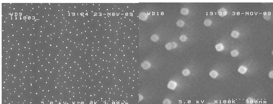
Figure 8 SEM images of salt particles from 3.5 wt% saltwater cone-jets at different magnifications.
