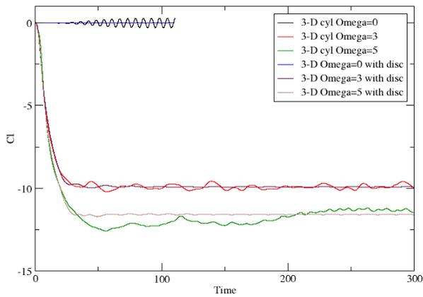
**Figure 12.** Mean lift coefficients for bare cylinder and cylinder with discs over a range of rotation numbers. Experimental measurements for bare cylinder, from Reid (1924).
