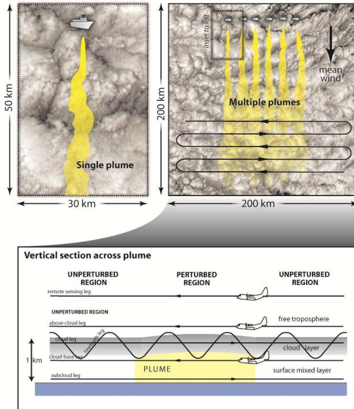
**Figure 13** A schematic of the plumes and the field experiment design
