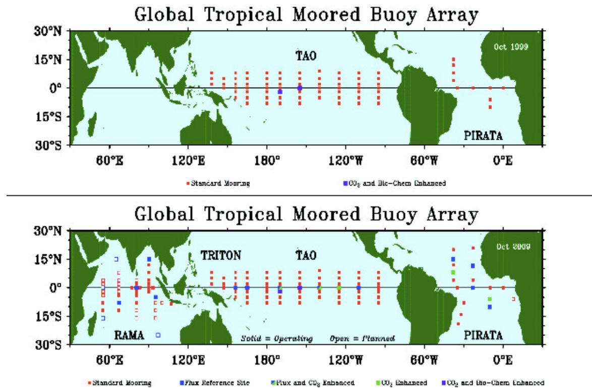
Figure 1: The evolving GT MBA over the past decades showing both existing and planned moorings to be completed over the next several years. The upper panel shows the arrays as they existed in 1999; the lower panel shows the arrays existing in 2009 plus planned additions.
