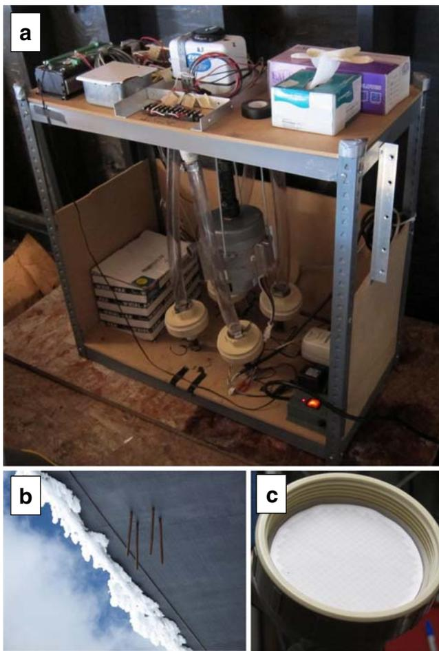
**Figure 1** Air sampling apparatus at the Mt. Bachelor Observatory. **a** A high-vacuum pump, electronics board and four separate filter housings were connected to intake pipes through holes at the base of the device. **b** Copper intake pipes emerged outside the building, facing into prevailing winds. **c** Polyethersulfone filter membrane (254 cm<sup>2</sup>, 0.8- $\mu$ m pores) inside plastic housing after an air sampling period
