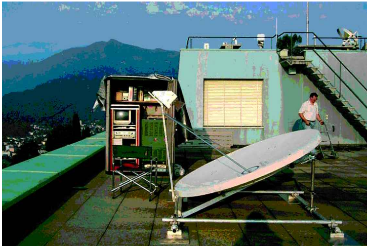
Figure 1. The University of Washington Orographic Precipitation Radar, OPRA, on the roof of the Swiss Meteorological Institute Osservatorio Ticinese in Locarno, Switzerland. The antenna has an offset feed and is set so the radar beam is pointing vertically. The radar's electronics, display and processing systems are contained within the small shelter to the left of the antenna.
