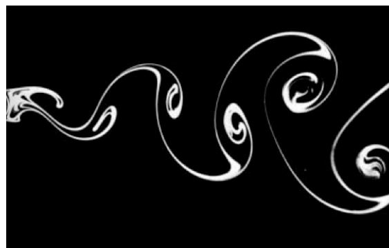
94. Kármán vortex street behind a circular cylinder at Re=140 . Water is flowing at 1.6 cm/s past a cylinder of diameter 1 cm. Integrated streaklines are shown by electrolytic precipitation of a white colloidal smoke, illuminated by a sheet of light. The vortex street is seen to grow in width downstream for some diameters. Photograph by Satoru Tanaka van Dyke, p. 56
